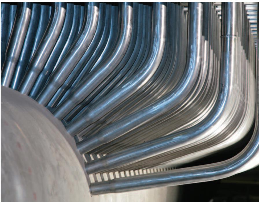
Application of boiler tubes during manufacturing of power plant equipment.
