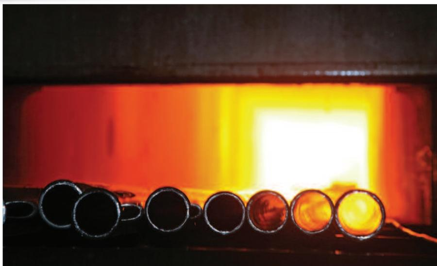
Tubes during the solution annealing process.
