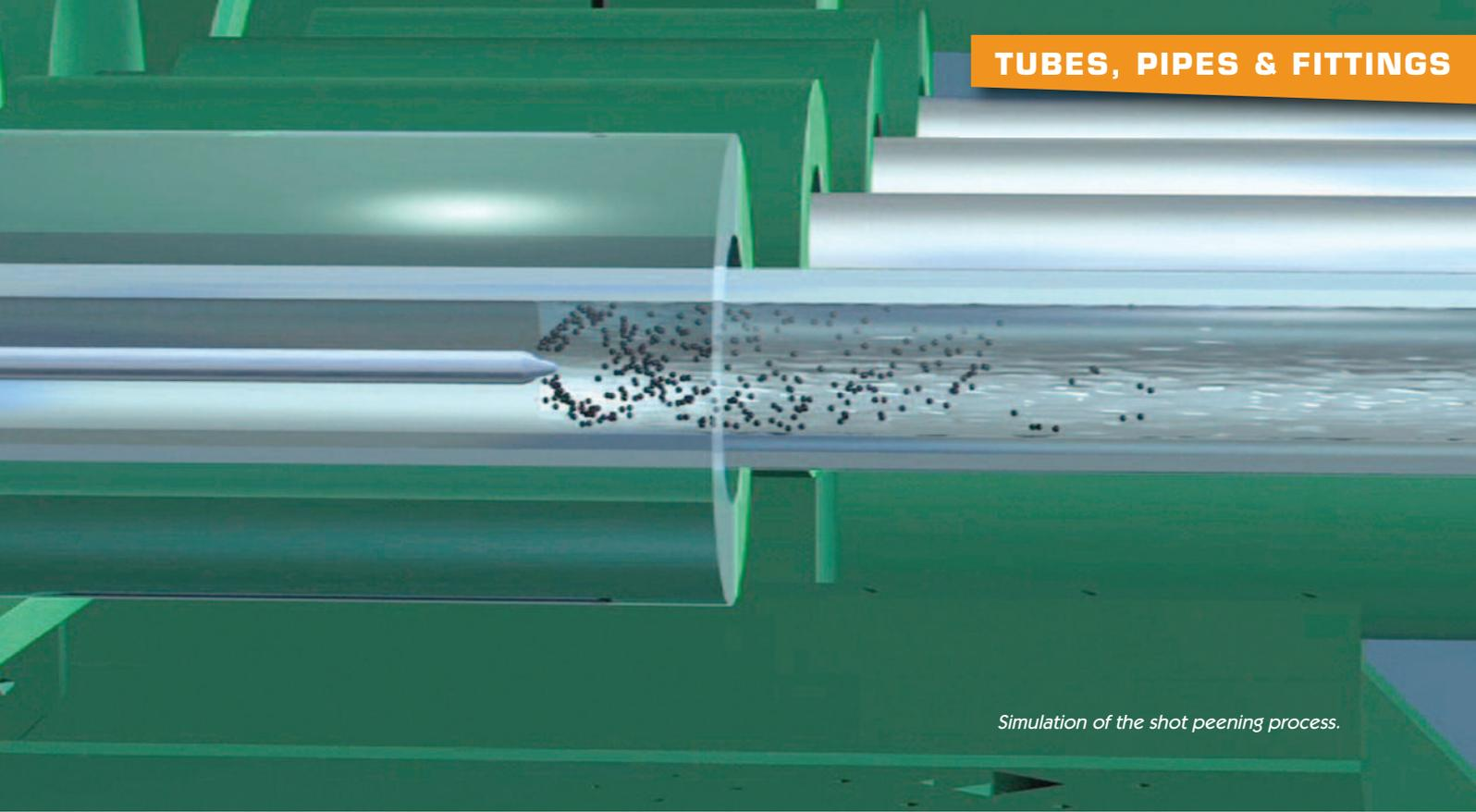
*Simulation of the shot peening process.*
