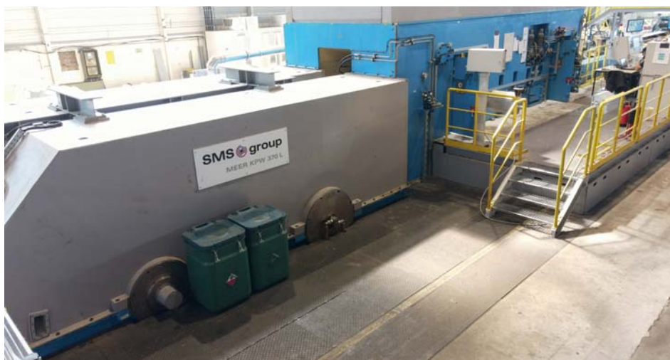
The addition of a cold pilger mill for large diameter tubes at the Remscheid, Germany plant has increased both capacity and capabilities.
