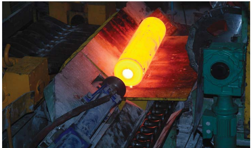
Hot extrusion is a critical process for determining the structure, quality, mechanical properties and ultimately length of a seamless tube or pipe.
