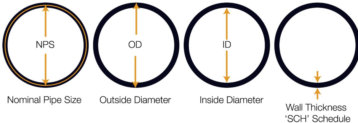
Nominal Pipe Size (NPS) originates from a North American set of standard sizes for pipes with the commonly used terminology of eg 2 inch, 4 inch, 6 inch etc having a historical association with the time when 'inch' referenced the actual ID.
